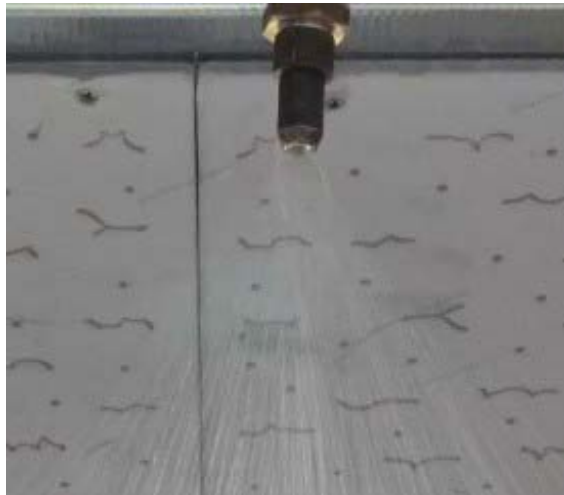
Figure 4. Water resistance test artificial rain nozzle
