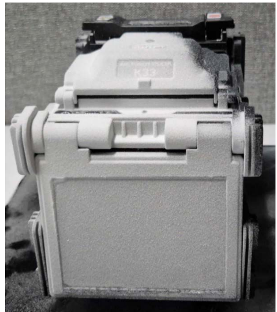
Figure 2.2. After dust test
