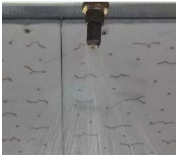
Figure 4. Water resistance test artificial rain nozzle
